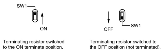
Figure 4-9 Switch Positions for Bus Terminating Resistors
